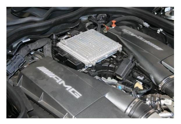
Remove the engine cover and disconnect the factory connectors from the ECU. The ECU pushes into rubber mounts and can be lifted directly up. Be gentle when handling the ECU and its associated wiring.
