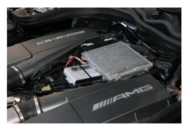
The Phase 1 tuning module can then sit in front of the factory ECU and be cable tied into place. There is freedom of mounting possible here with the Phase module also able to be located in the valence panel for easy access.
