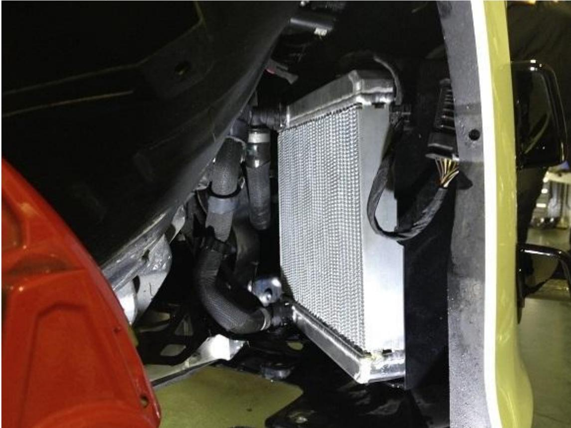
Snap the hoses back into place on the new intercooler connectors, and the rest of the mechanical installation is a reversal of the existing procedure.
