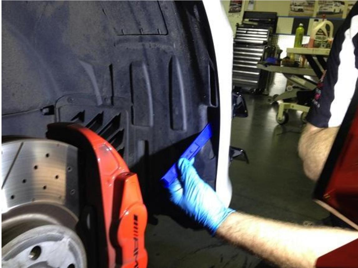
The other trim clip that you need to remove is located here. This completes the process of removing the trim clips, so now you can get on with swapping the intercooler proper.
