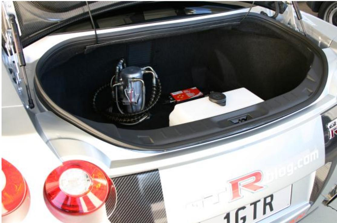
Mounting the tank assembly is recommended in the left hand side (close to centre) of the trunk compartment. This will allow you to run the stainless braided lines up and under the car through the existing hole in the GTR floor-pan in this location. Some modification of the rubber bung in the floor may be required, or even simpler is to remove it altogether.
