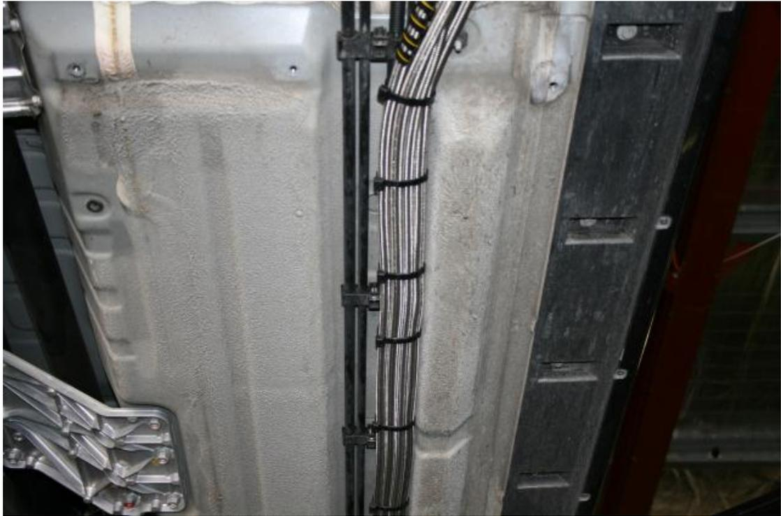
There is ample room for the WR35FS fuel lines to run along the side of the existing fuel lines that are installed on the GTR from factory. These lines can be tied together as shown in the picture to keep the lines nicely located and in position.
