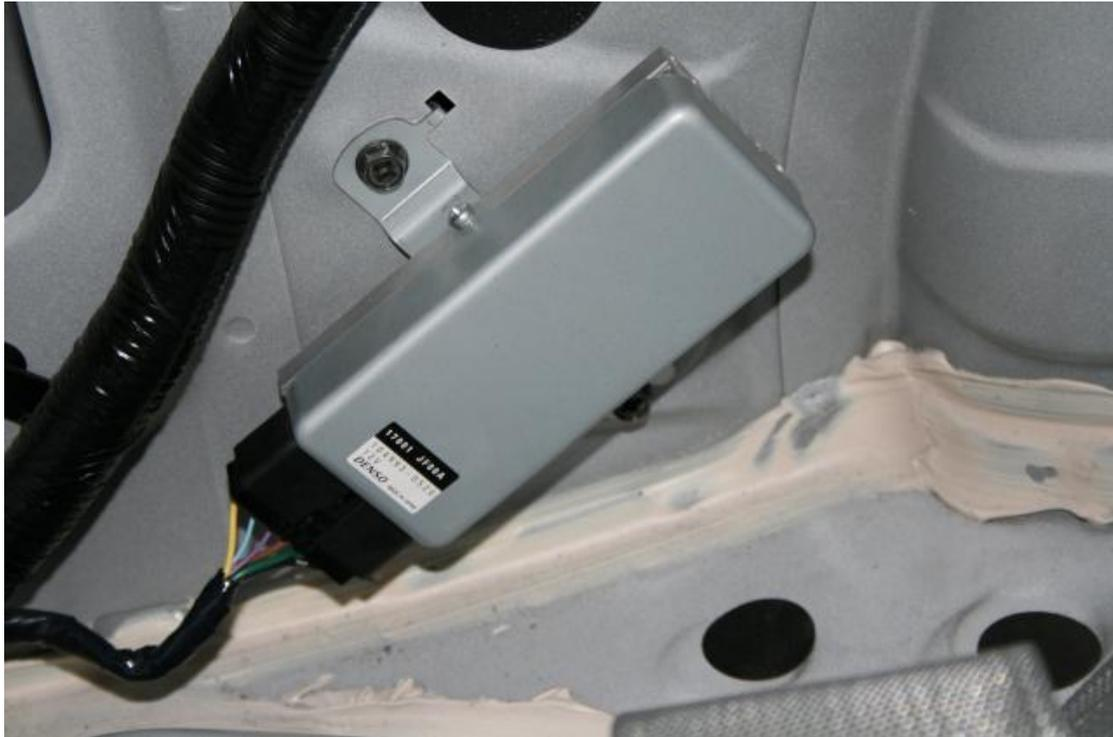
Wiring the WR35FS fuel system is a straightforward process with all of the system wiring being laid out logically. The two trigger wires for the system which are green and brown need to be tapped into the existing green and brown trigger wires on the Fuel Pump Control Module. Locating the Fuel Pump Control Module requires the trim to be removed on the RHS inner B pillar.
