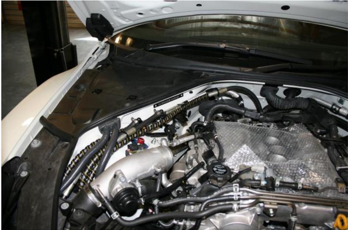
Each of the WR35FS fuel system lines will be marked with a naming label when you receive the system. This makes it easy to identify the lines when you have run them into the engine bay as shown in this picture.
