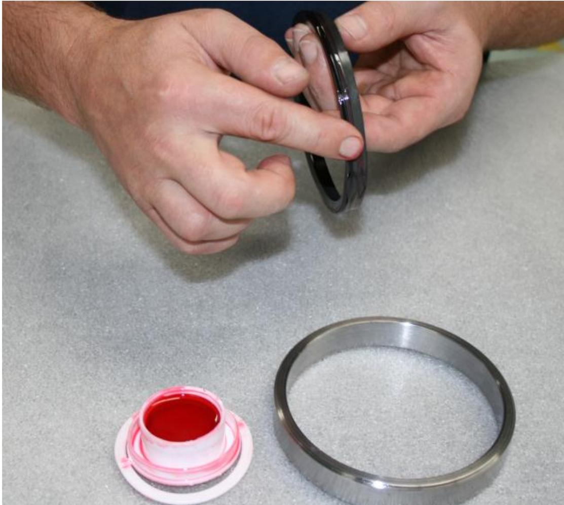
WR35PS must be specifically lubricated before installation is carried out. This lubrication must be the same type as the transmission. In the instance of using WR35TM in the transmission then please thoroughly wipe the O-ring surface using WR35TM as shown.
