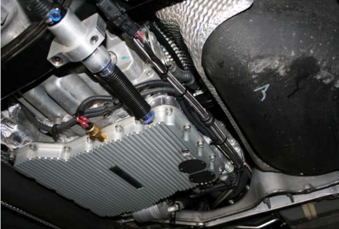
The feed line for the transmission cooler then runs down alongside the billet sump as pictured here. Use the supplied cable ties to strap the feed line up nice and tight, ensuring it doesn't rub against anything else.
