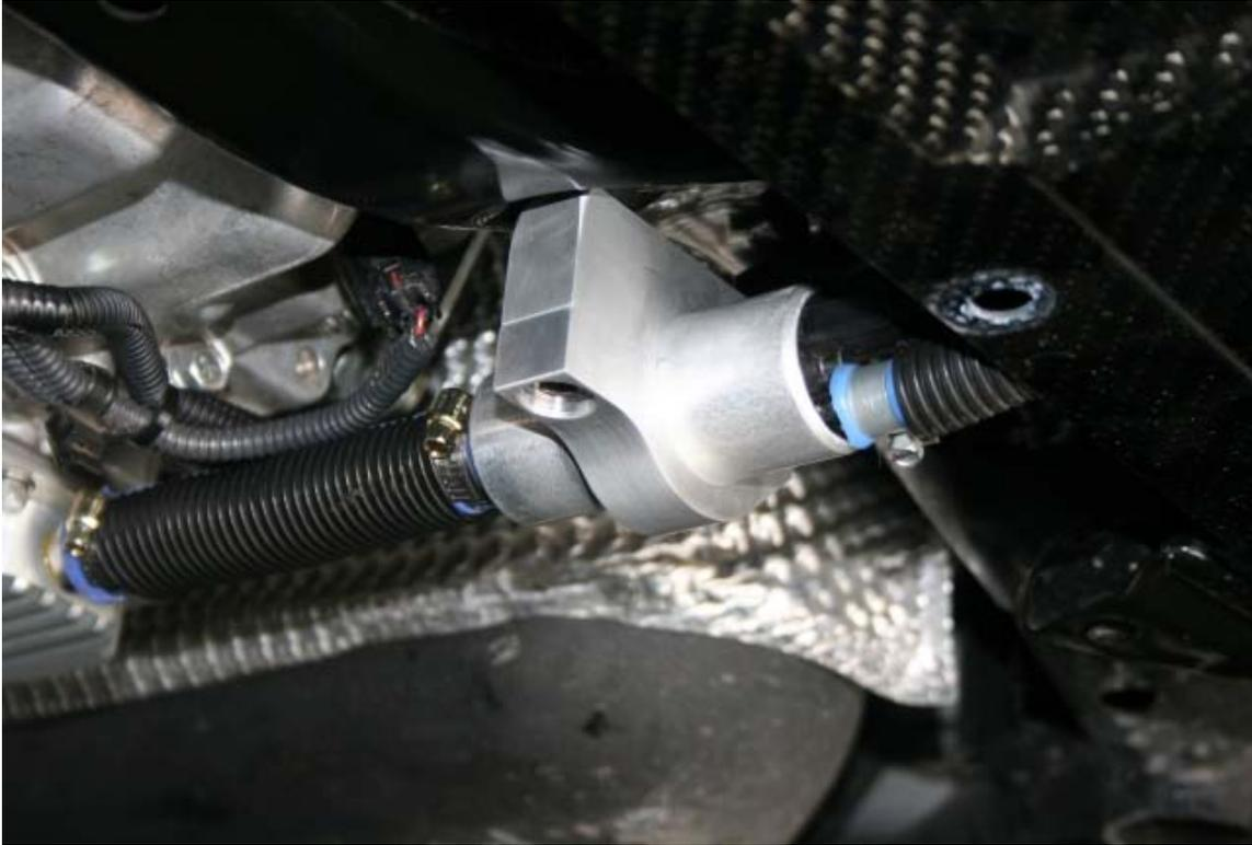
The Silicone hose that attaches to both the inlet and outlet of the WR35TC pump assembly has been covered in black plastic for these photographs but the orientation of the pump and bracket is still clearly obvious. A long bolt is supplied to mount the bracket through a factory mounting hole.
