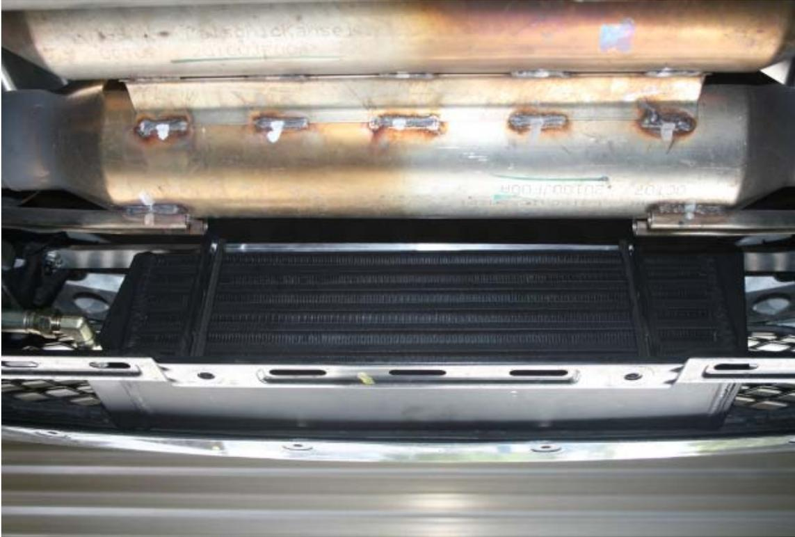
WR35TC Intercooler mounted in place between the exhaust system and the rear grille. Note that this Mkl version of the cooler has a bottom entry, where later production models have both top entry and exit for the tanks.
