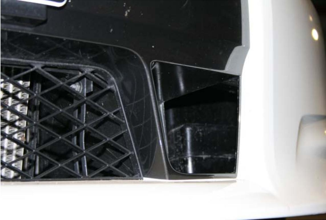
The air vent needs to have its back cutout to match the opening on the other side of the front bar for the oil cooler. This is a simple job that you can undertake with a sharp blade. Ensure you do this slowly and don't slip or mark the bodywork!
