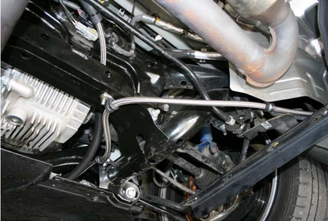
There is sufficient length in the feed and drain lines for the WR35TC intercooler to allow for custom placement if need be, and individual routing of the fluid lines around the existing exhaust system assembly.
