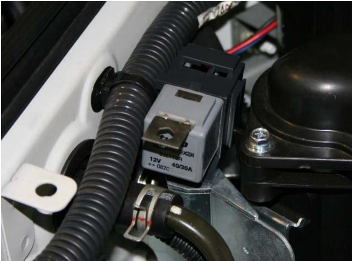
Tuck the supplied relay in under the battery cover for secure mounting.
