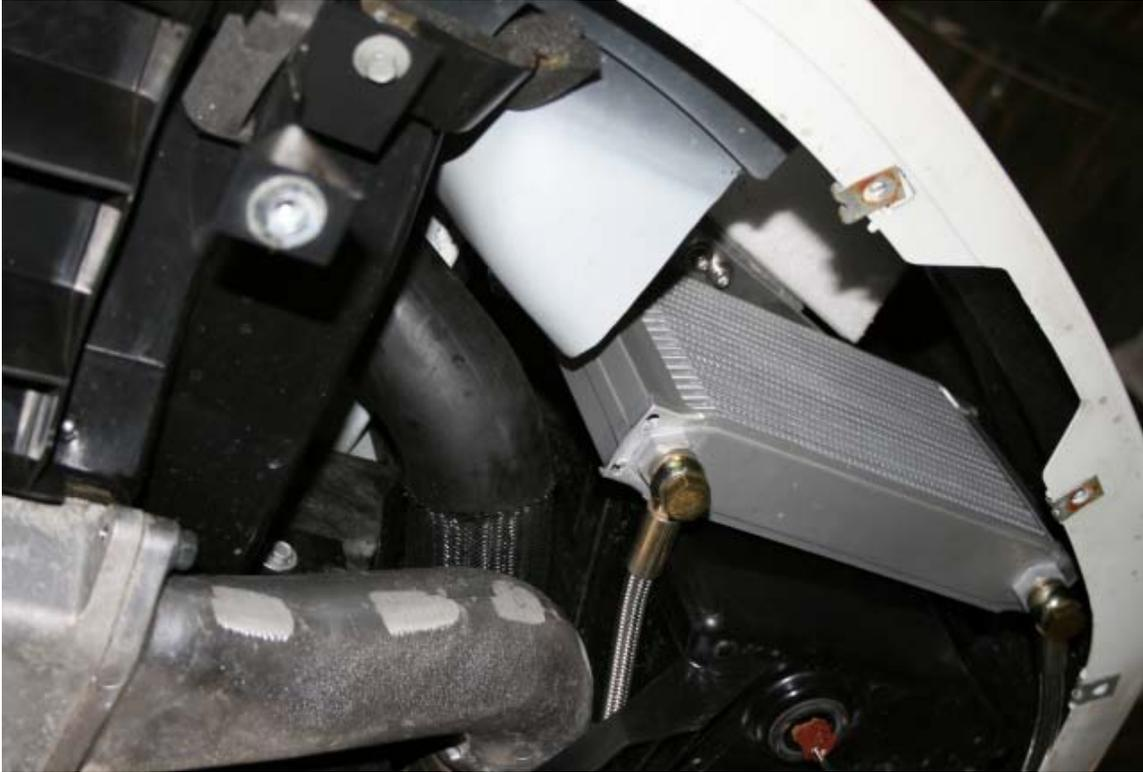
Line the cooler up so that it sits directly at the outlet of the air duct for the cleanest and coolest flow of air.
