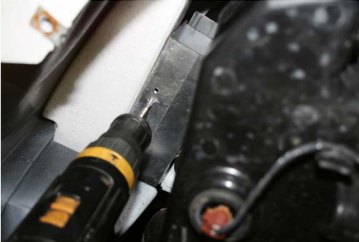
Line up the holes in the mounting bracket on the intrusion bar (use a marking pen) and then drill the holes using the supplied 6.9mm drill bit. Once the holes are drilled they can then be tapped with the supplied tap.
