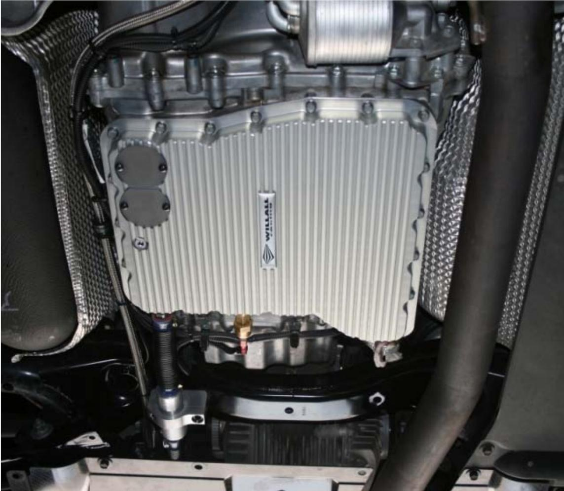
WR35TC finned aluminium sump bolts directly in place of the factory pressed tin item. The magnets need to be removed from the original sump and placed in the WR35TC sump, as does the drain plug and tube assembly.
