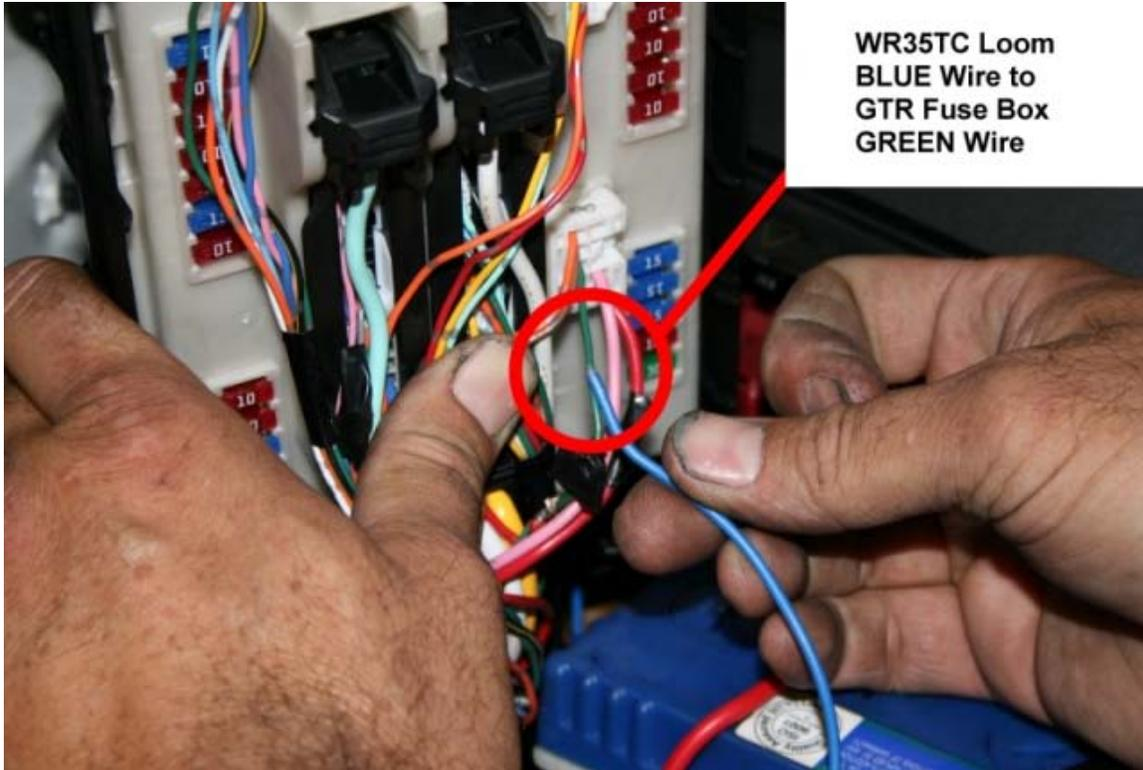
The supplied wiring loom needs to be connected to the GTR fuse-box (located by the battery) as follows. The blue wire from the WR35TC loom needs to be connected to the green wire as shown.
