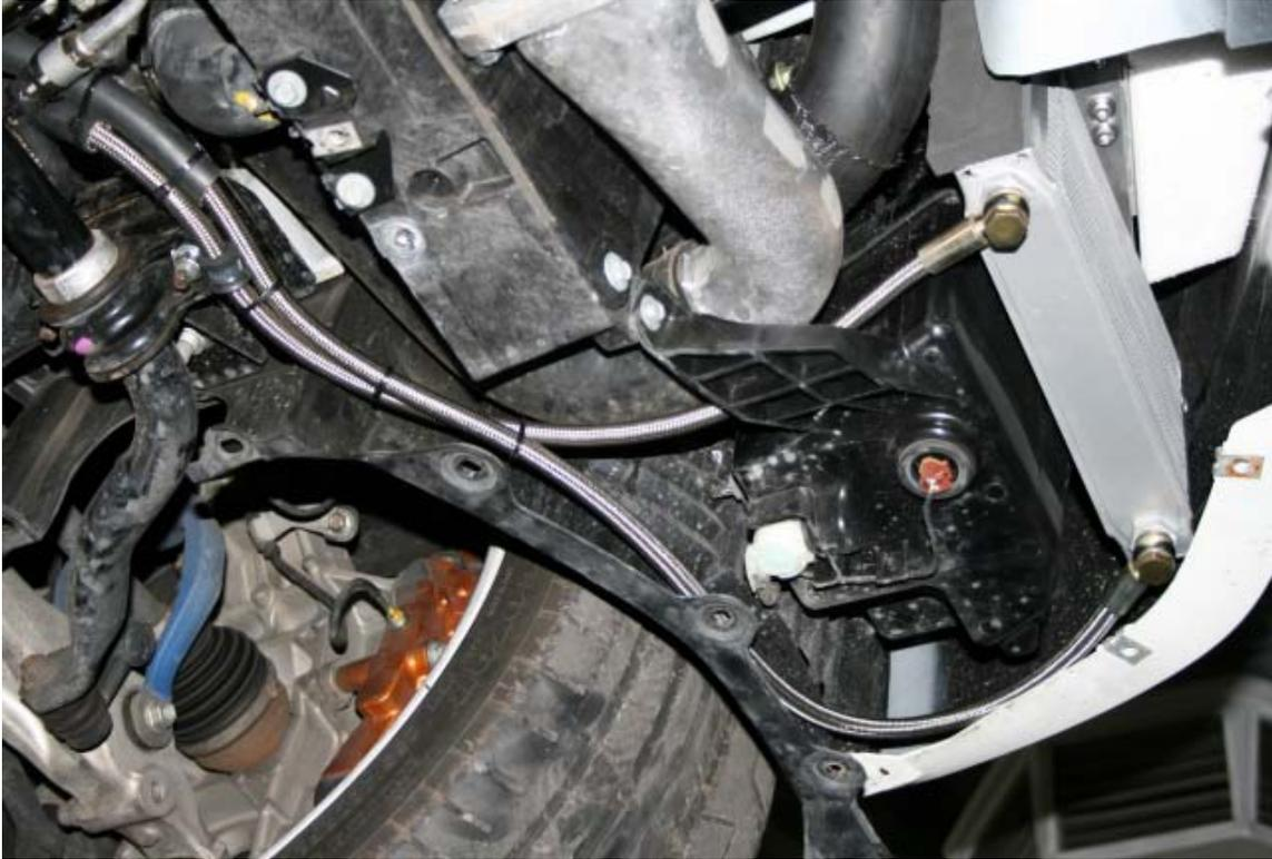
Run the lines to the cooler and back to the transmission, but ensure that wherever they can touch against any other component that the supplied sheathing is used (can be different to pictured) to protect against abrasion damage
