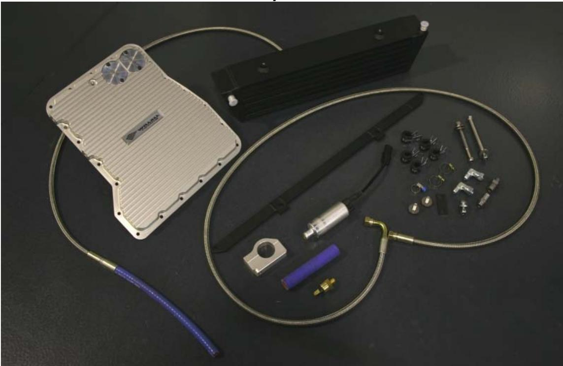
WR35TC GR6 Transmission Cooler components laid out for visual inspection. WR35TC is comprehensive but also logical in its layout and installation.
