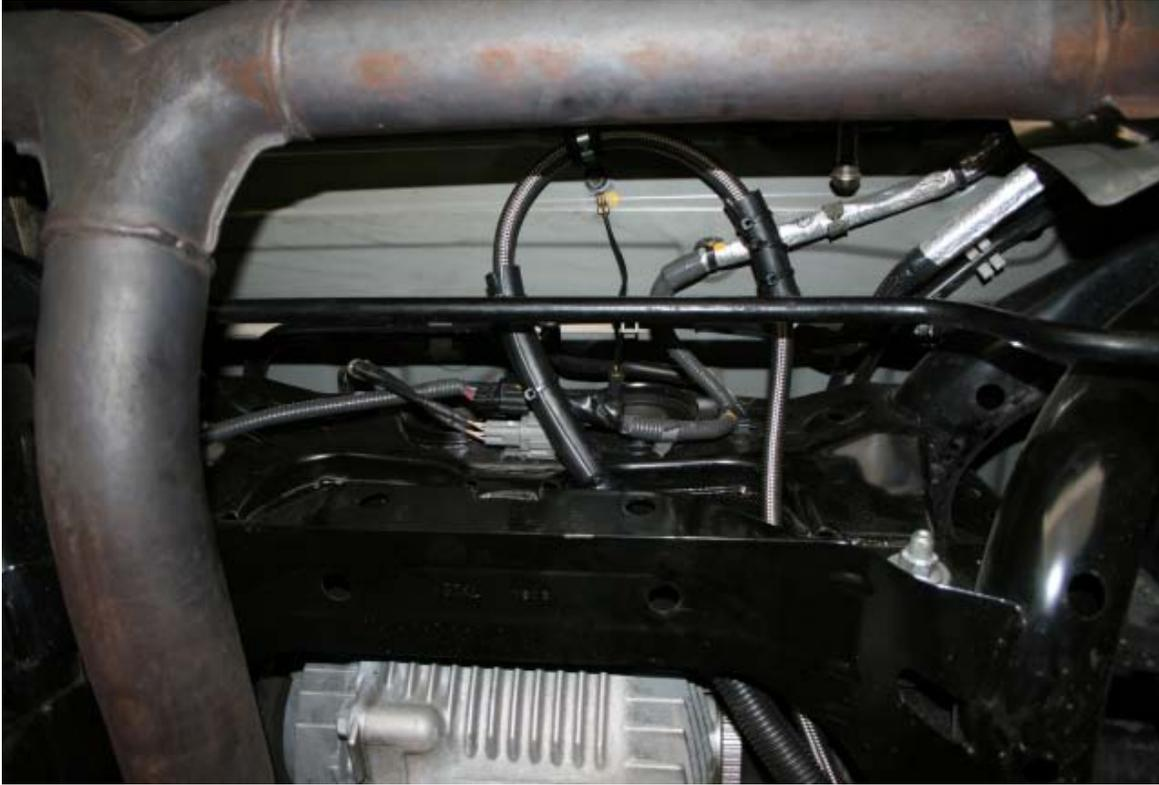
The main transmission fluid feed line from the back of the pump loops around at the back of the car as shown here. Use a supplied P clamp off the earth point for the wiring and make sure the bend is open and flowing to avoid any kinks in the line.
