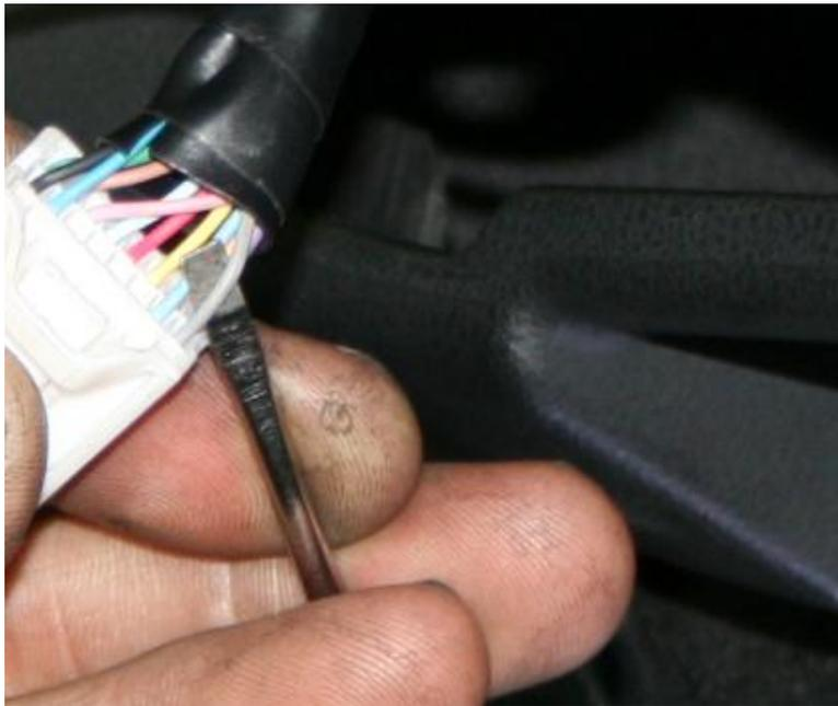
If installing a WR35WS version that utilises the existing washer tank then this is the washer motor trigger wire when unplugged from the indicator stork. It is the grey wire
