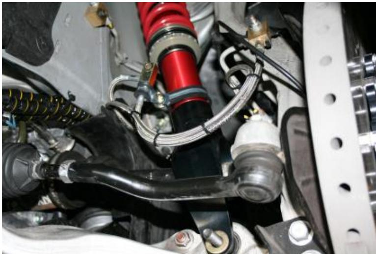
WR35WS spray nozzle lines can then be cable tied to the existing brake lines so that their shape emulates that of the brake lines perfectly. Use cable ties at similar distances to that show in the photograph.
