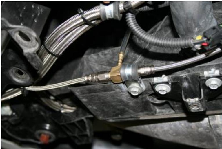
The braided spray nozzle lines can now be run to the shown location on the bottom of the radiator shroud where a hole exists in the structure for fitment of a supplied P-clamp. The rubber line can
