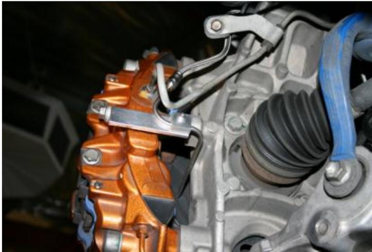
Mounting the water spray brackets requires removal of the caliper bolt in the centre of the front caliper. It is easy to locate and remove. The process is the same for the left and right hand sides of the vehicle.
