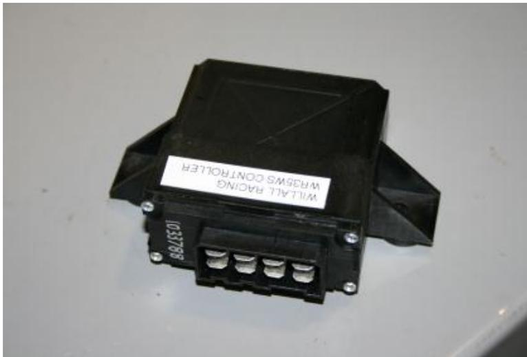
Once the system is wired the control module (which is pre-programmed not to trigger the WR35WS system under 40mph) can be tucked away neatly under the dash, ensuring there is no strain on the wiring.
