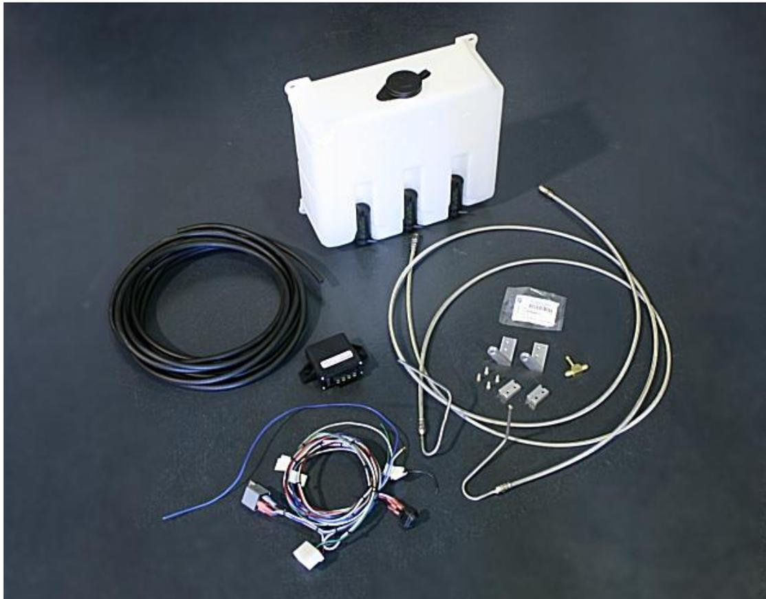
WR35WS is a specially designed brake cooling system that uses water as a means of directly cooling the GTR brakes. Capable of reducing brake temperatures by up to 100 degrees WR35WS also has the advantage of extending brake component life. Installation is straight forward but should be carried out referencing the pictorial installation guide
