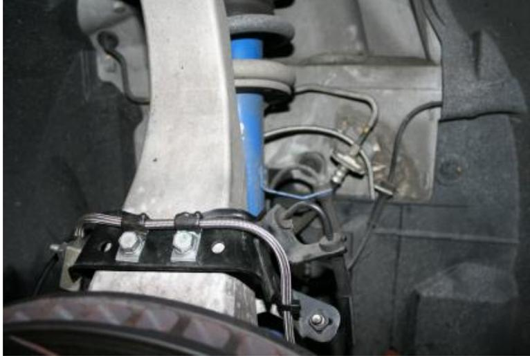
Use P-clamps (if supplied in earlier systems) to fix the spray nozzle lines to the front mounting point as show in the picture or simply route the braided line underneath the black metal factory bracket. This ensures that there will be no fouling between the suspension, brake, wheel and any WR35WS component.
